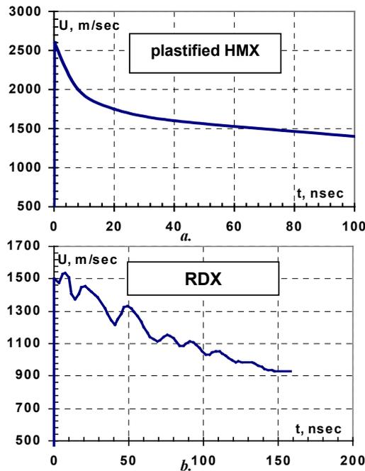
**FIGURE 2. PARTICLE VELOCITY PROFILES FOR: (a) PLASTIFIED (98,5% TMD) HMX AND (b) RDX (93% TMD).**
