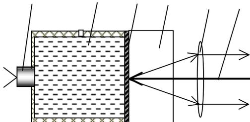
1 - detonator; 2 - liquid HE in cylindrical cell or sample of solid HE; 3 - Al covering ( $\sim 1 \mu\text{m}$ ) or Al foil (5-10  $\mu\text{m}$ ); 4 - crystal of LiF; 5 - laser beam ( $\lambda=694.3 \text{ nm}$ ); 6 - focusing lens.
