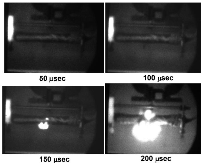
**FIGURE 6. CORDIN IMAGES OF TUBE FAILURE FOR PS-1.**
