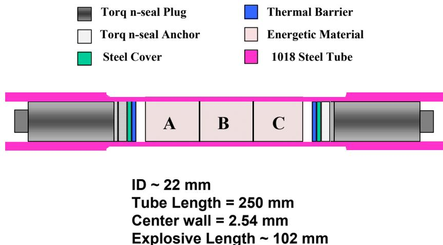
**FIGURE 1. SCHEMATIC OF SMALL-SCALE COOKOFF EXPERIMENT.**
