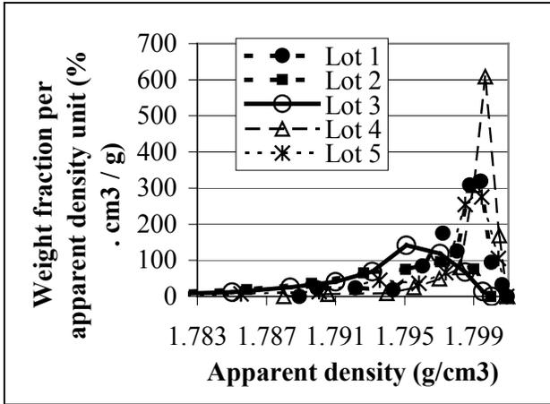
**Figure 2 : Apparent density distribution of commercial grade RDX**
