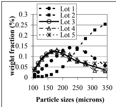
**Figure 1 : Particle sizes of commercial grade RDX**
