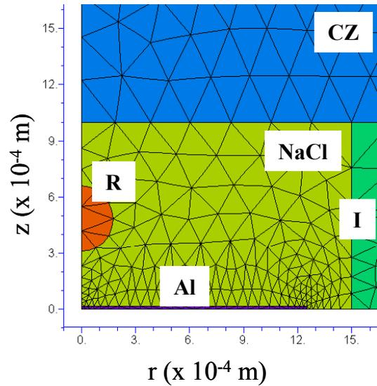
**FIGURE 3: VIEW OF INPUT STRUCTURE FOR FLEXPDE SIMULATIONS. SEE TEXT FOR MATERIAL ABBREVIATIONS.**
