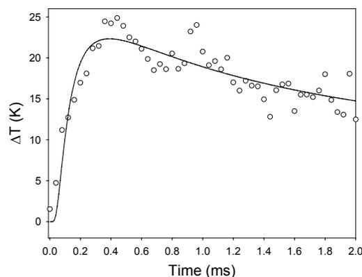
**FIGURE 7: 1-D ANALYTICAL FIT (LINE) TO THERMAL WAVE DATA (CIRCLES) FOR NaCl AT 0.05 GPa.**
