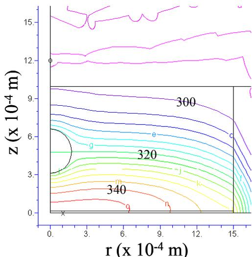
**FIGURE 4: SNAPSHOT OF ISOTHERMS IN NaCl CALCULATED BY FLEXPDE 300  $\mu$ S AFTER THERMAL WAVE INITIATION.**
