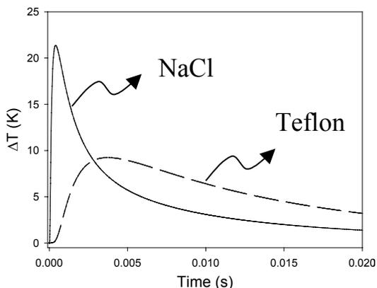
**FIGURE 8: SIMULATIONS OF THE PROGRESSION OF A THERMAL WAVE IN NaCl (SOLID) AND TEFLON (DASHED).**
