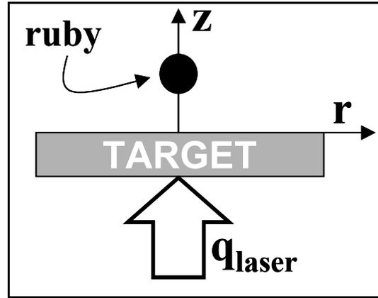
**FIGURE 2: CARTOON REPRESENTING 1-D ANALYTICAL MODEL OF HEAT FLOW.**
