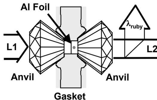
**FIGURE 1. VIEW OF THE EXPERIMENTAL ANVIL CELL.**
