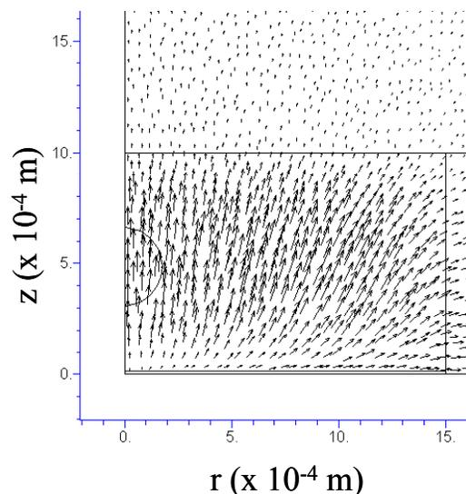
**FIGURE 5: SNAPSHOT OF DISPLACEMENT VECTORS CALCULATED BY FLEXPDE 300  $\mu$ S AFTER THERMAL WAVE INITIATION.**
