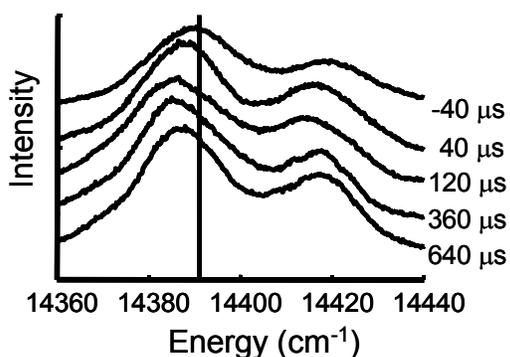
**FIGURE 6: TIME-RESOLVED RUBY FLUORESCENCE SPECTRA EXHIBITING THE PROGRESSION OF A THERMAL WAVE VIA ENERGY SHIFTS IN ITS EMISSION LINES.**
