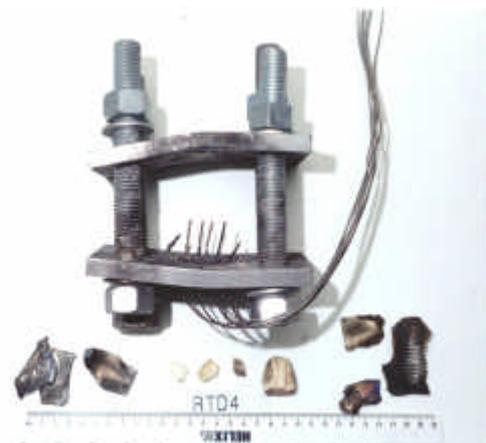
**FIGURE 10: TYPICAL REMAINS FROM RDX/TNT EXPERIMENT**
