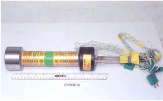
**FIGURE 1: PREPARED BURNING TUBE**
