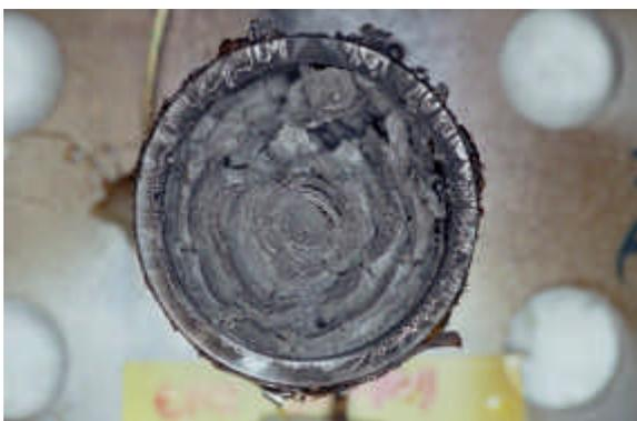
**FIGURE 14: RESIDUE FROM 'CIGAR BURN' OF RDX/HTPB 85:15 IN GLASS-WINDOWED VEHICLE**
