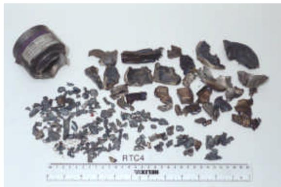
**FIGURE 8: VEHICLE REMAINS FROM PARTIALLY-HEATED RDX/TNT EXPERIMENT**
