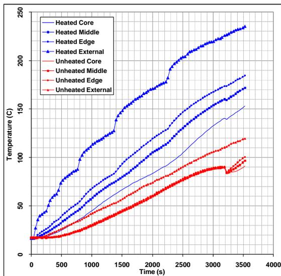
**FIGURE 9: TEMPERATURE HISTORY OF PARTIALLY HEATED RDX/TNT EXPERIMENT**
