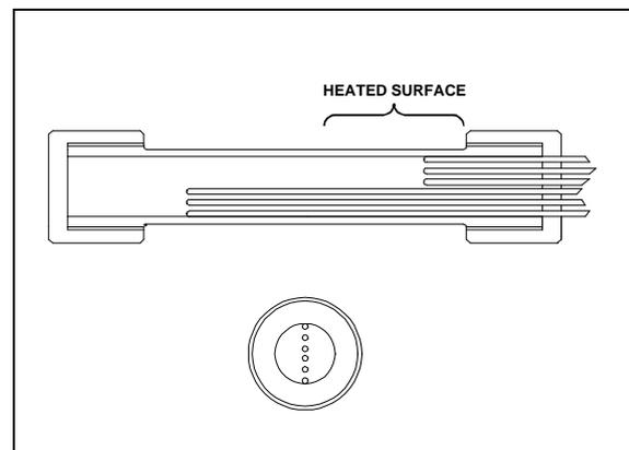
**FIGURE 3: SKETCH OF PARTIALLY HEATED BURNING TUBE SHOWING THERMOCOUPLE ARRANGEMENT**
