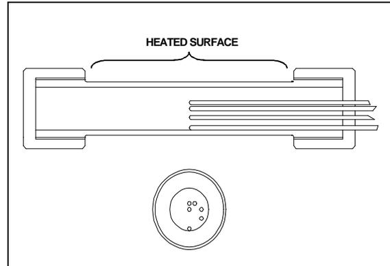
**FIGURE 2: SKETCH OF FULLY HEATED BURNING TUBE SHOWING THERMOCOUPLE ARRANGEMENT**
