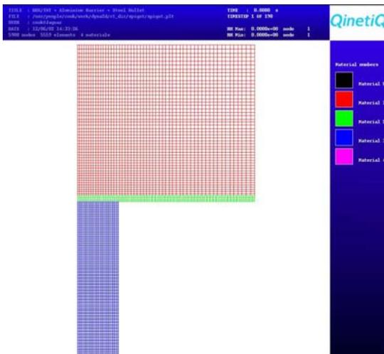
**FIGURE 2. DYNA2D MESH OF A FRAGMENT IMPACT SIMULATION.**
