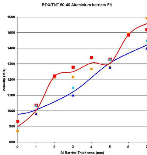
**13.15MM DIAMETER STEEL PROJECTILES AGAINST RDX/TNT CHARGES COVERED BY ALUMINIUM BARRIERS. THE EXPERIMENTAL RESULTS ARE SHOWN IN RED AND THE CALCULATED VALUES IN BLUE**
