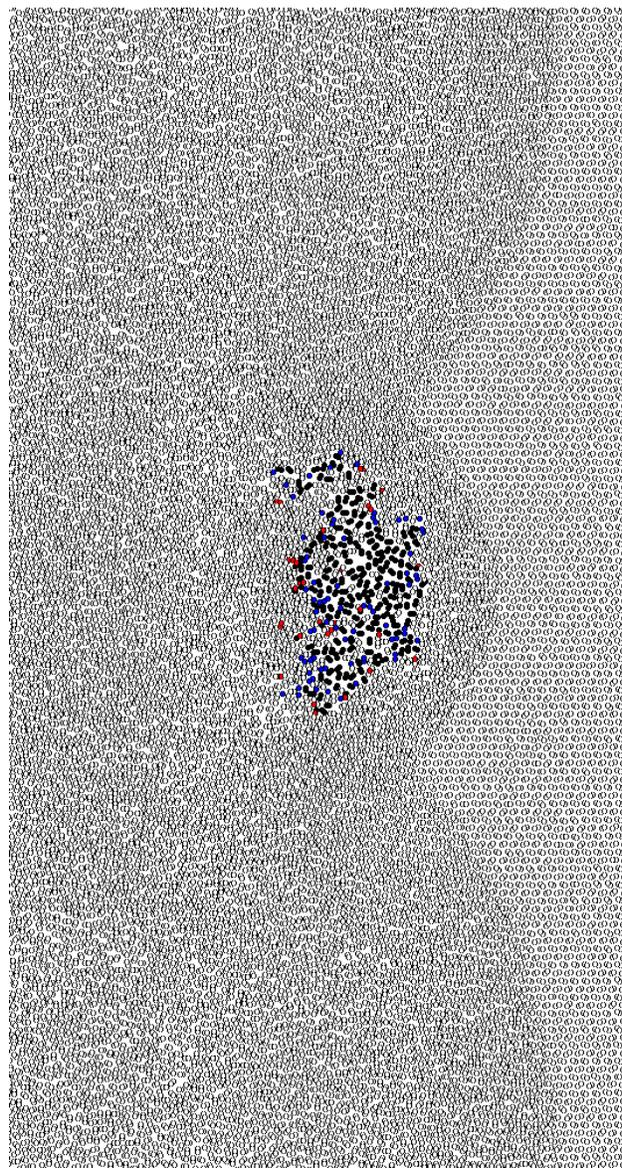
**FIGURE 5. SAME AS FIGURE 3, 6.87 PS AFTER IMPACT. BLACK MOLECULES ARE  $A_2$  OR  $B_2$  PRODUCTS; RED AND BLUE ATOMS REPRESENT FREE RADICALS OR MANY-BODY REACTION COMPLEXES.**
