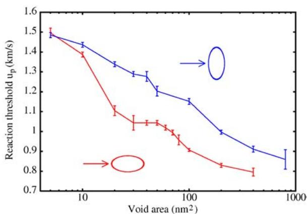
**FIGURE 7. SHOCK STRENGTH (IN TERMS OF PARTICLE VELOCITY  $u_p$ ) REQUIRED TO INITIATE CHEMICAL REACTIONS FOLLOWING COLLAPSE OF ELLIPTICAL VOIDS OF VARIOUS SIZES AND ORIENTATIONS.**
