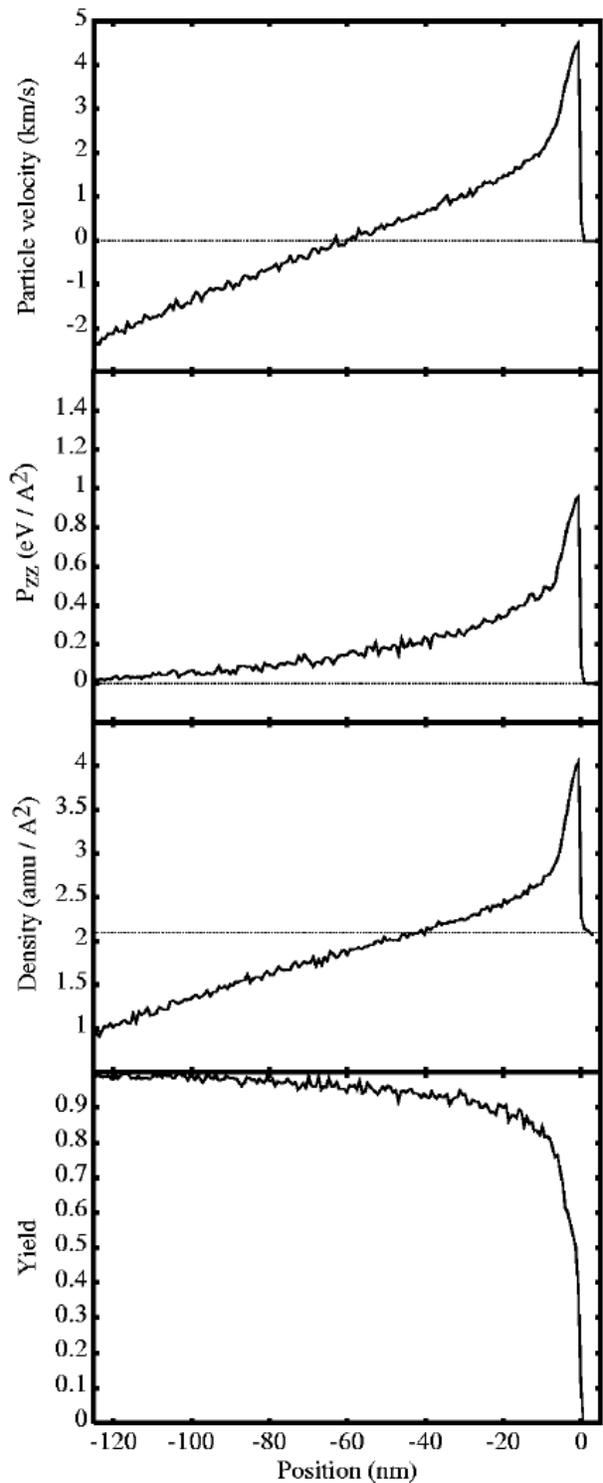
**FIGURE 2. 2-D UNSUPPORTED DETONATION PROFILES. THE (PERIODIC) CROSS-SECTION IS 124 NM WIDE AND THE ENTIRE SAMPLE CONTAINS 234,200 ATOMS. YIELD IS DEFINED AS THE FRACTION OF ATOMS IN PRODUCT ( $A_2$  OR  $B_2$ ) MOLECULES.**
