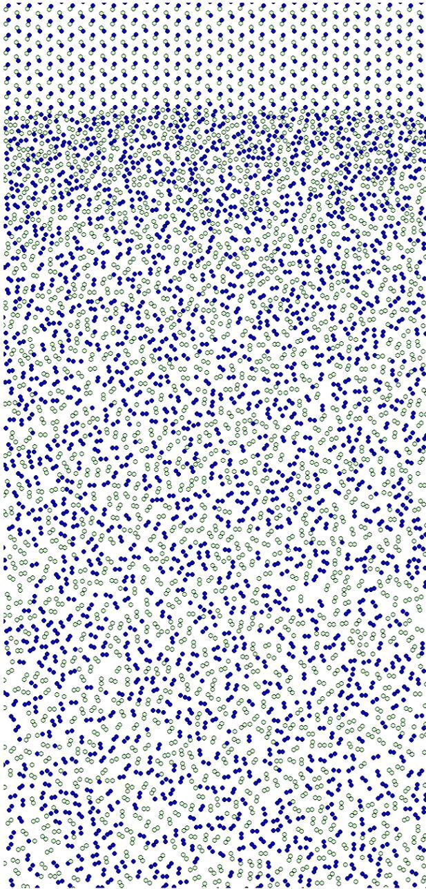
**FIGURE 1. UNSUPPORTED DETONATION WAVE TRAVELING FROM BOTTOM TO TOP IN A TWO-DIMENSIONAL AB SOLID INITIATED BY A THIN INERT  $A_2$  FLYER PLATE IMPACT. THE ATOMS ARE COLORED ACCORDING TO THEIR IDENTITY (EITHER A OR B). PERIODIC BOUNDARY CONDITIONS ARE APPLIED IN THE TRANSVERSE DIRECTION.**
