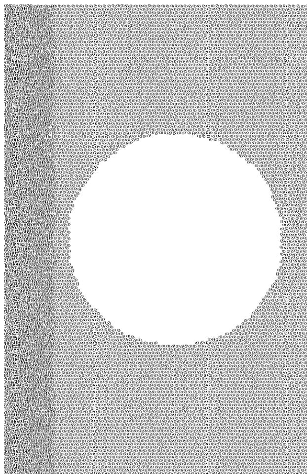
**FIGURE 3. SUPPORTED NONREACTIVE SHOCK WAVE (WITH PARTICLE VELOCITY  $u_p = 1.38$  KM/S) APPROACHING A 20 NM DIAMETER VOID, 0.25 PS BEFORE IMPACT. ONLY A CLOSE-UP PORTION OF THE ENTIRE (129 NM X 45 NM) SIMULATION CELL ARE SHOWN IN THIS AND FOLLOWING FIGURES.**
