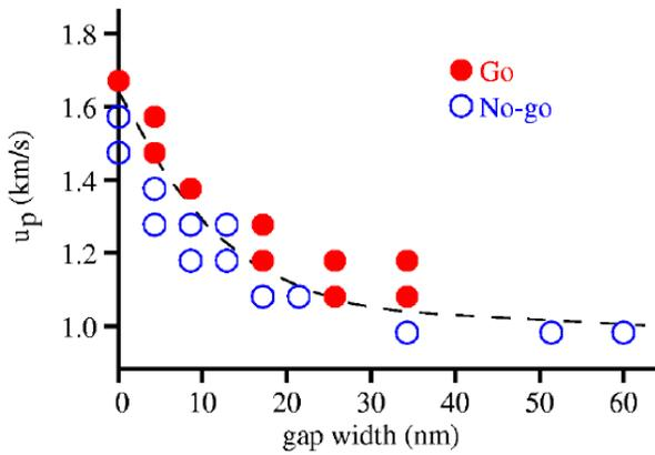
**FIGURE 8. SHOCK STRENGTH (IN TERMS OF PARTICLE VELOCITY  $u_p$ ) REQUIRED TO INITIATE CHEMICAL REACTIONS ACROSS VARYING GAP WIDTHS.**
