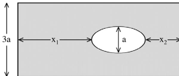
**FIGURE 6. SIMULATION GEOMETRY USED FOR TWO-DIMENSIONAL ELLIPTICAL VOID STUDIES.**
