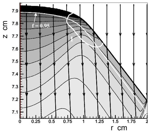
**FIGURE 8B. PRESSURE CONTOURS AND STREAMLINES FOR  $a = 0.1 \mu\text{s}^{-1}$  AND  $n = 1.0$**
