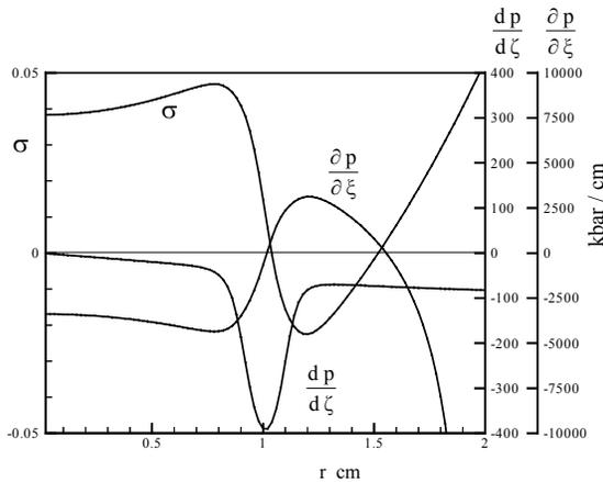
FIGURE 5B. NEGATIVE THERMICITY IN RADIALLY GRADED EXPLOSIVES
