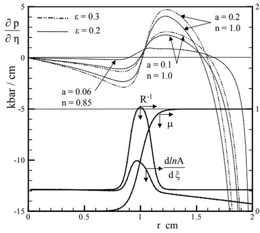
**FIGURE 5A.  $\partial p/\partial \eta$  IN A RADIALLY GRADED EXPLOSIVE FOR DIFFERENT REACTION RATES**
