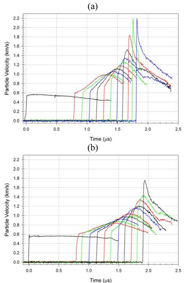
**FIGURE 3. EFFECT OF DENSITY ON WAVE PROFILES. PARTICLE VELOCITY WAVE PROFILES FOR SHOT 1162 (a) (MATERIAL A, 1.826 g/cm<sup>3</sup>) AND SHOT 1164 (b) (MATERIAL B, 1.830 g/cm<sup>3</sup>). THE INPUT STRESS IS NEARLY IDENTICAL  $3.89 \pm 0.03$  GPa IN BOTH EXPERIMENTS.**
