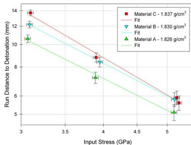
**FIGURE 6. POP-PLOTS FOR THREE DIFFERENT DENSITY NEW PBX 9501 MATERIALS.**
