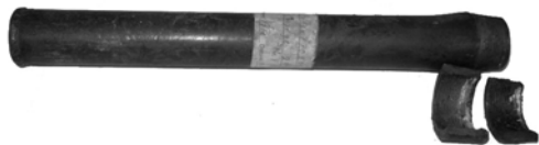
FIGURE 7. TEST TUBE AFTER THE DETONATION TEST.
