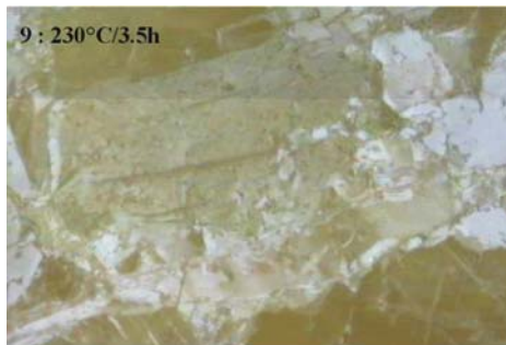
Figure 10: TATB heated at 230°C during 3 h and 30 mn then cooled - Disappearing of intragranular porosity by creation of recrystallisation domains (white zones on the figure)
