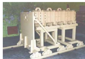
Figure 6: Samples recovering system associated to CEG Deimos gas launcher
