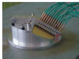
Figure 4: TATB-based target instrumented by pins array
