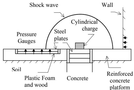
**FIGURE 8 - EXPERIMENTAL SET-UP FOR CYLINDRICAL CHARGE TESTS (SIDE VIEW)**
