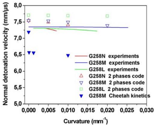
FIGURE 3 -  $D_n - \kappa$  CURVES FOR G258, 3" TEST CYLINDER.
