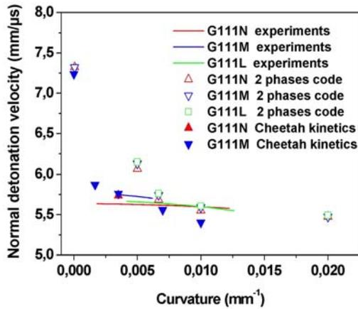
FIGURE 2 -  $D_n - \kappa$  CURVES FOR G111, 3" TEST CYLINDER.
