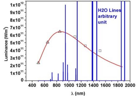
FIGURE 7 - TYPICAL EXAMPLE OF SPECTRUM FITTING FOR G258N.
