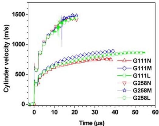
**FIGURE 4 - CYLINDER TEST VELOCITIES MEASURED USING VISAR.**
