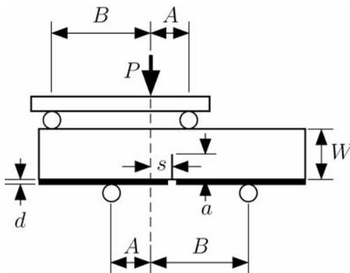
Figure 2 Asymmetric beam loading
