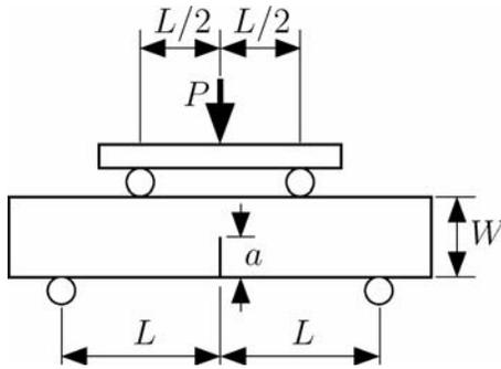
Figure 1 Symmetric beam loading
