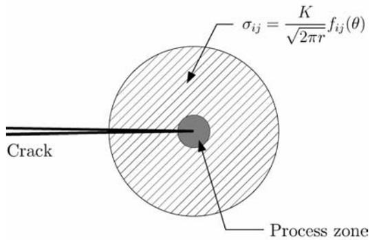
**Figure 9 Idealized fracture configuration from conventional brittle fracture mechanics.**
