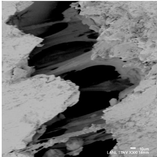
**Figure 10 Electron micrograph shows taffy like binder bridging fracture surfaces.**
