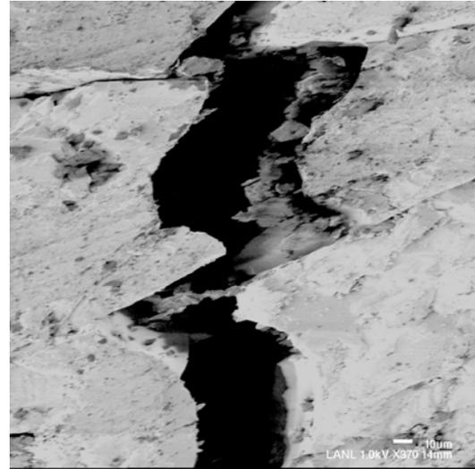
**Figure 11 Electron micrograph shows fracture of crystalline HMX.**
