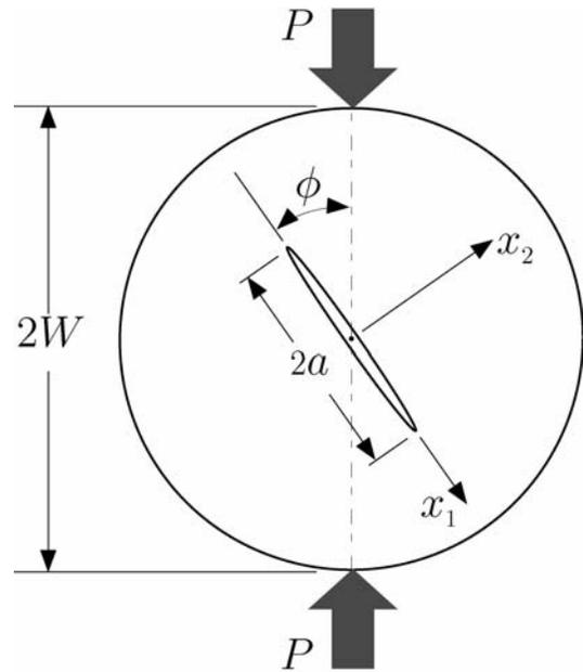
Figure 4 Brazil geometry with initial flaw
