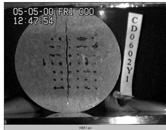
Figure 5 Frame from movie of conventional Brazil test
