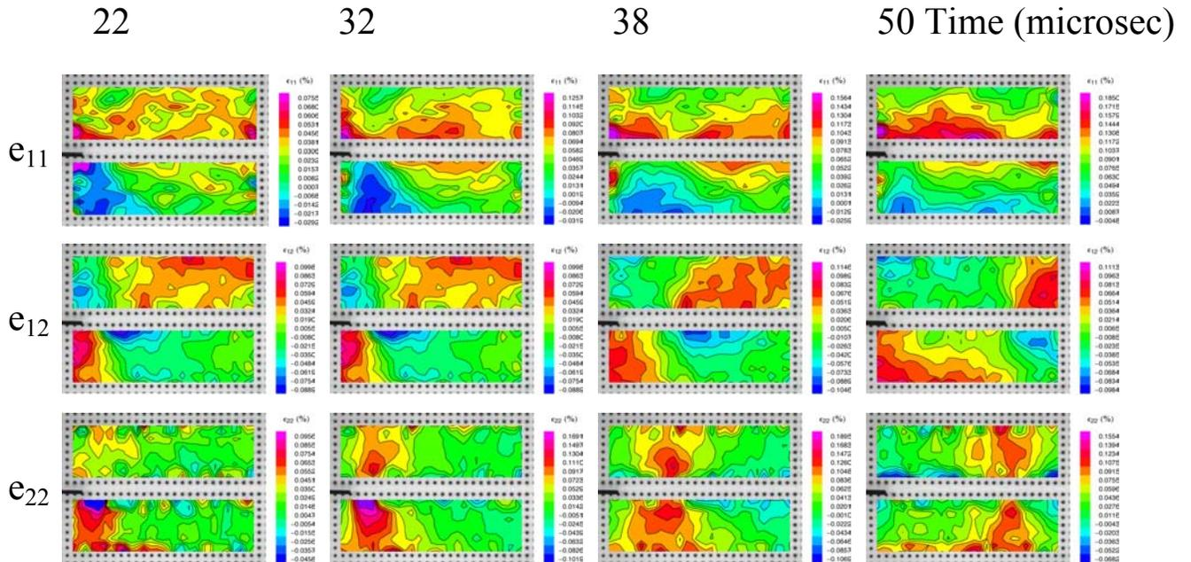
Figure 17 Contour plots of strain fields derived from digital image correlation, at a sequence of times, provide the basic information about the conditions around the bridging zone and crack tip.
