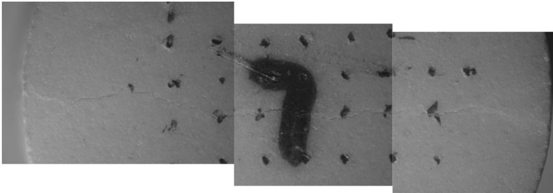
Figure 16 Optical micrograph of fracture across a Brazil sample shows the erratic path and wedge features at loading regions typical of these samples.
