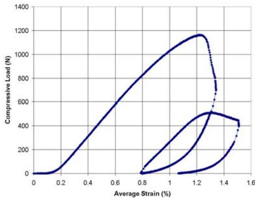
**Figure 7 Cyclic loading in Brazil test shows changes in stiffness as crack develops.**
