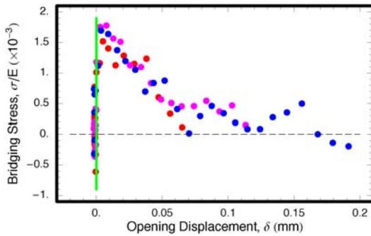
**Figure 12 Bridging Stress Law quantifies the amount of bridging stress depending on separation of fracture surfaces.**
