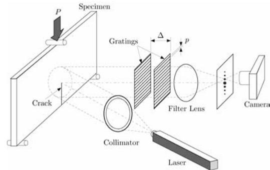
**Figure 8 Coherent Gradient Sensing (CGS) test configuration.**
