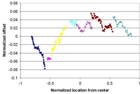
Figure 15 Offset from nominal centerline of crack path expressed as a fraction of the diameter.
