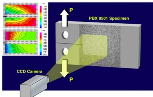
Figure 3 Modified compact tension
