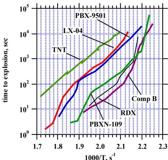
**FIGURE 4. ODTX DATA FOR SEVERAL HMX AND RDX FORMULATIONS**
