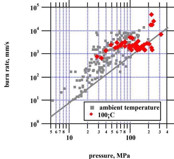
**FIGURE 10. BURN RATE DATA FOR COMP B, CALCULATED FROM BURN WIRES, FOR INITIAL TEMPERATURE OF 100°C**
