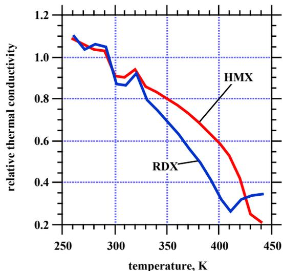
**FIGURE 2. RELATIVE CHANGE IN THERMAL CONDUCTIVITY OF HMX AND RDX WITH TEMPERATURE, NORMALIZED TO AMBIENT TEMPERATURE VALUE**
