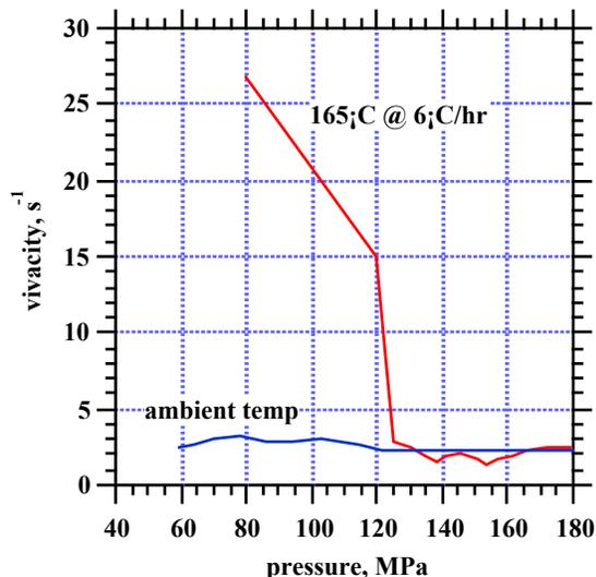
FIGURE 14. TYPICAL VIVACITY DATA FOR PBXN-109 AT AMBIENT AND ELEVATED TEMPERATURES
