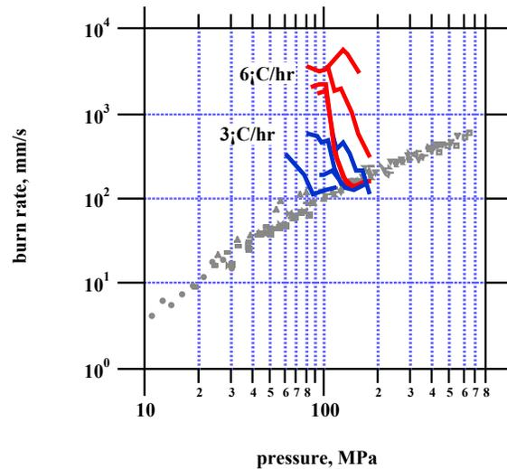
**FIGURE 12. DEFLAGRATION RATE DATA FOR PBXN-109, CALCULATED FROM BURN WIRES, FOR SAMPLES HEATED TO 165-185°C**
