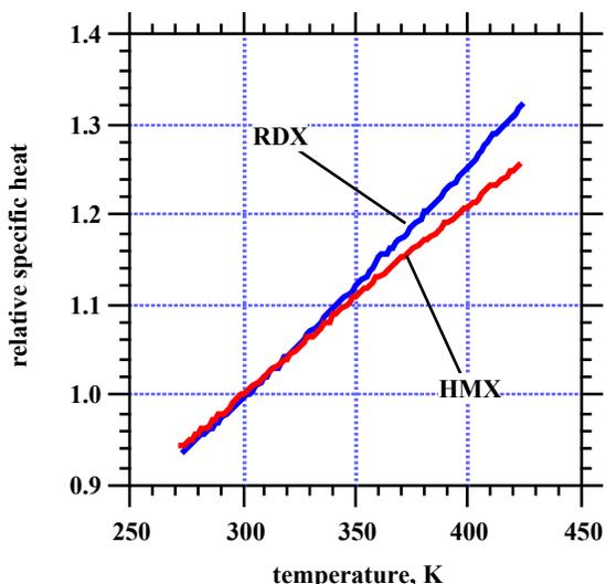
**FIGURE 3. RELATIVE CHANGE IN SPECIFIC HEAT,  $C_p$ , OF HMX AND RDX WITH**
