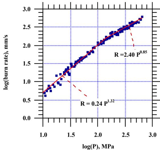
**FIGURE 11. BURN RATE DATA FOR PBXN-109, CALCULATED FROM BURN WIRES,**
