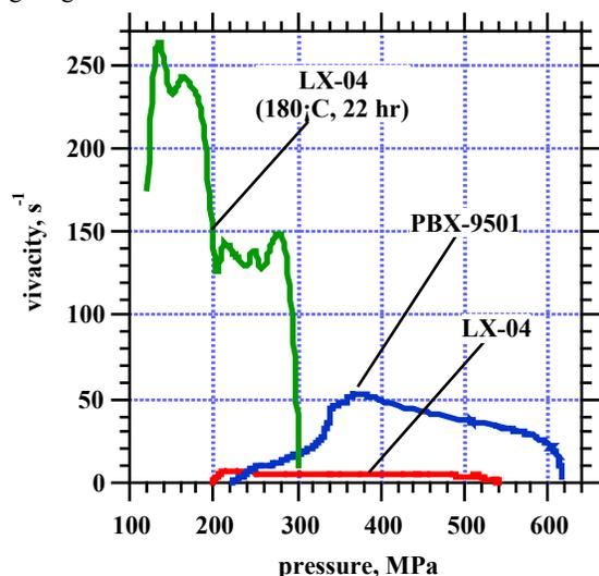
**FIGURE 6. VIVACITY DATA FOR TWO HMX FORMULATIONS AT AMBIENT AND ELEVATED TEMPERATURES**
