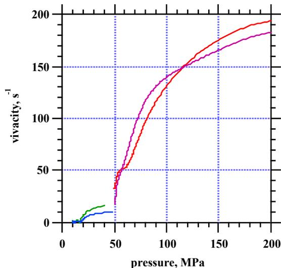
**FIGURE 9. VIVACITY DATA FOR COMPOSITION B, SHOWING RESULTS FROM TWO RUNS AT 10 MPa AND 50 MPa INITIAL PRESSURES**
