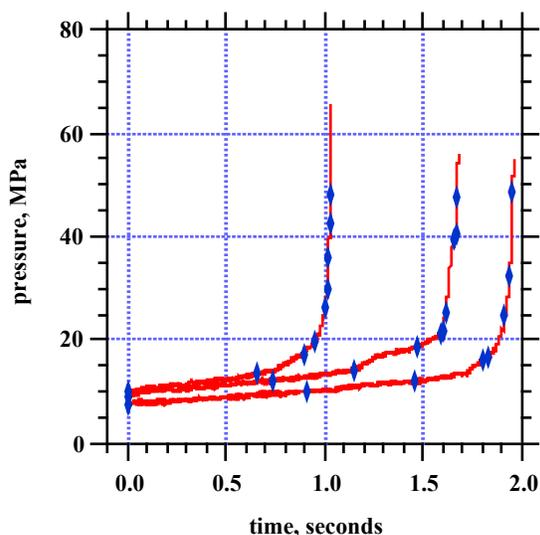
**FIGURE 7. PRESSURE-TIME DATA FROM DEFLAGRATION OF COMPOSITION B, SHOWING SLOW INITIAL BURN FOLLOWED BY RAPID (DECONSOLIDATIVE) BURNING. SYMBOLS INDICATE EMBEDDED WIRE SIGNALS.**
