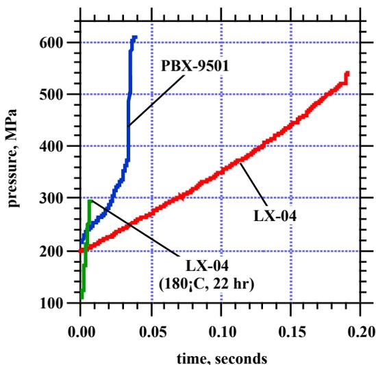
**FIGURE 5. PRESSURE DATA FROM DEFLAGRATION OF TWO HMX FORMULATIONS AT AMBIENT AND ELEVATED TEMPERATURES**
