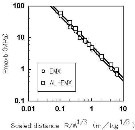
**FIGURE 10. RELATION BETWEEN PEAK BUBBLE PULSE PRESSURE AND SCALED DISTANCE**
