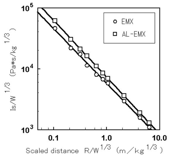
**FIGURE 6. RELATION BETWEEN SCALED SHOCK WAVE IMPULSE AND SCALED DISTANCE**
