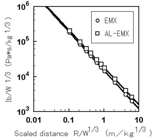
**FIGURE 11. RELATION BETWEEN SCALED BUBBLE PULSE IMPULSE AND SCALED DISTANCE**
