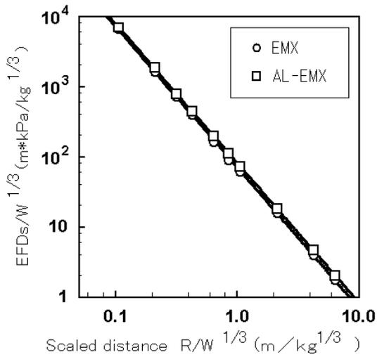
**FIGURE 7. RELATION BETWEEN SCALED SHOCK ENERGY FLUX DENSITY AND SCALED DISTANCE**
