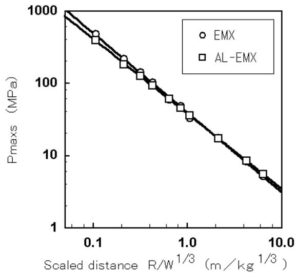
**FIGURE 5. RELATION BETWEEN PEAK SHOCK WAVE PRESSURE AND SCALED DISTANCE**
