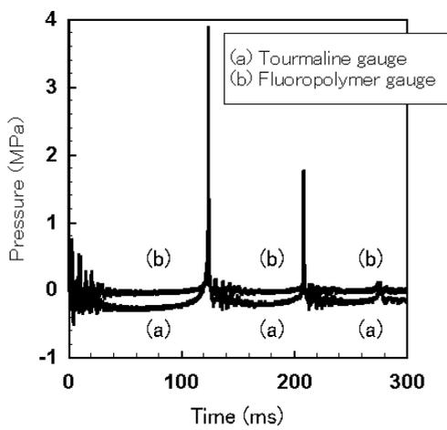
**FIGURE 8. EXAMPLE OF BUBBLE PULSE PROFILE**
