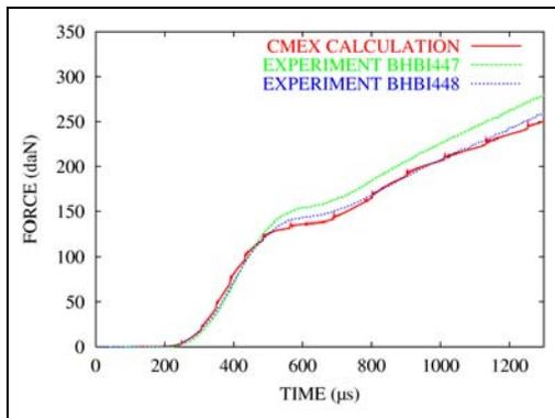
**FIGURE 9. EXPERIMENTAL AND NUMERICAL FORCES IN BRAZILIAN TEST**
