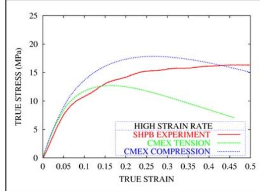
**FIGURE 7. COMPARISON OF SHPB EXPERIMENT AND CMEX RESULTS- CMEX RESULT IN TENSION**
