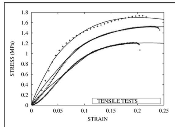
**FIGURE 6. EXPERIMENTAL (points) AND NUMERICAL (solid lines) RESULTS ON TENSILE TESTS FOR B2211D**
