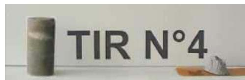
**FIGURE 3. CUMULATIVE DAMAGE AFTER TWO IMPACTS (SHOT 4/99) (left: after first impact, right: plug after second impact)**
