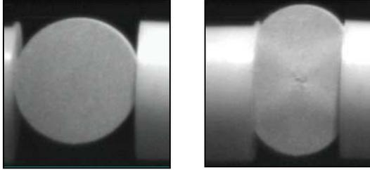
**FIGURE 4. PHOTOGRAPHS OF DYNAMIC BRAZILIAN TEST (left: initial , right: first failure)**
