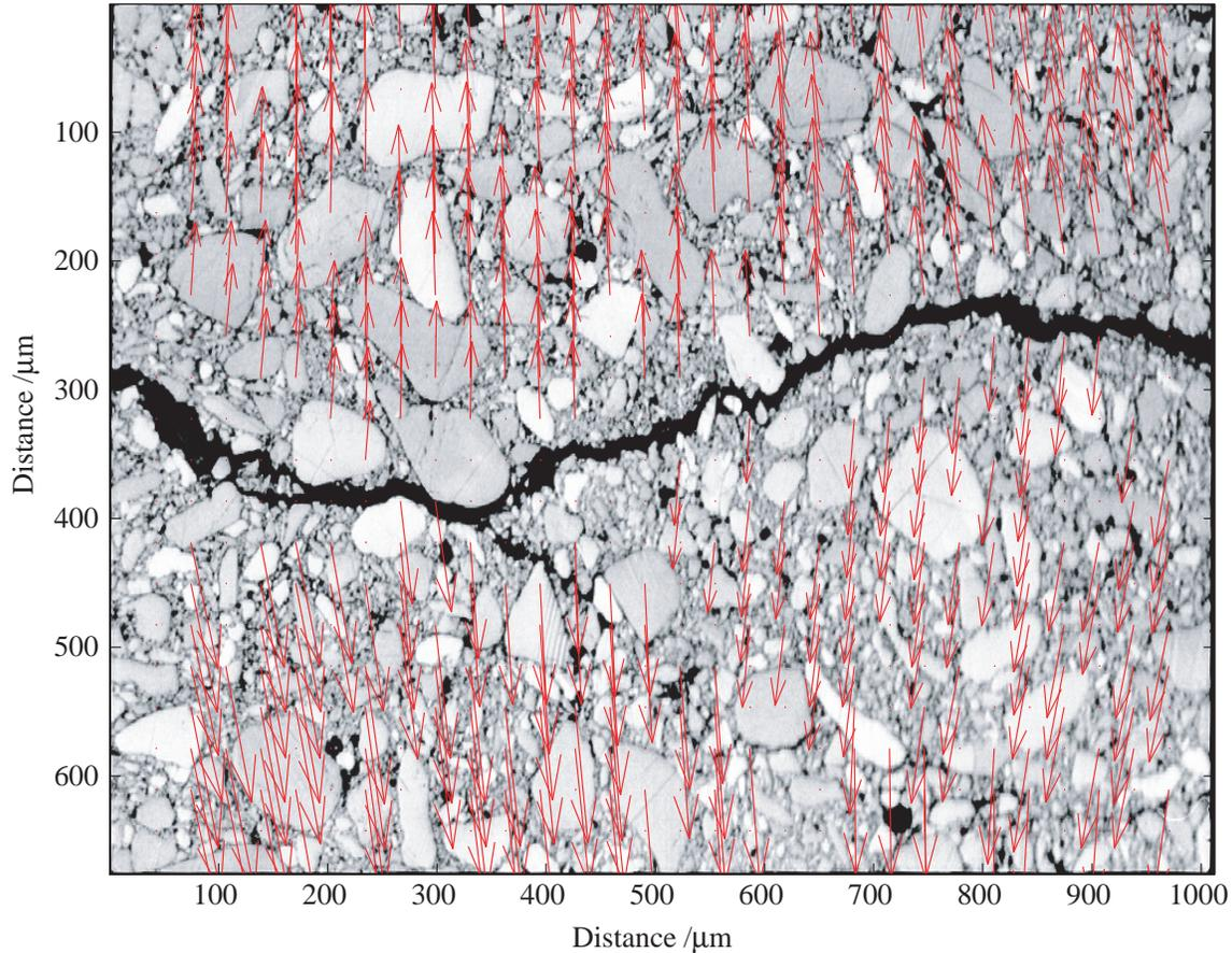
**FIGURE 2: EDC 37 LOADED TO FAILURE DURING A DICC TEST. THE VECTORS INDICATE THE AVERAGE DISPLACEMENT MEASURED AT EACH SUB-IMAGE.**
