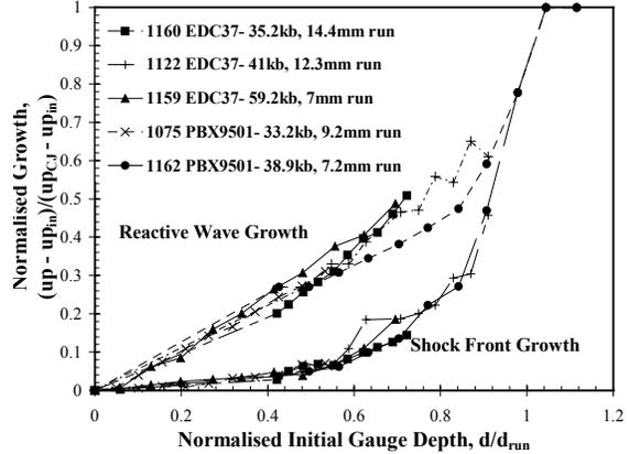
**FIGURE 8. COMPARES THE NORMALISED RATE OF GROWTH OF THE SHOCK AND THE REACTIVE WAVE IN EDC37 WITH PBX9501.**
