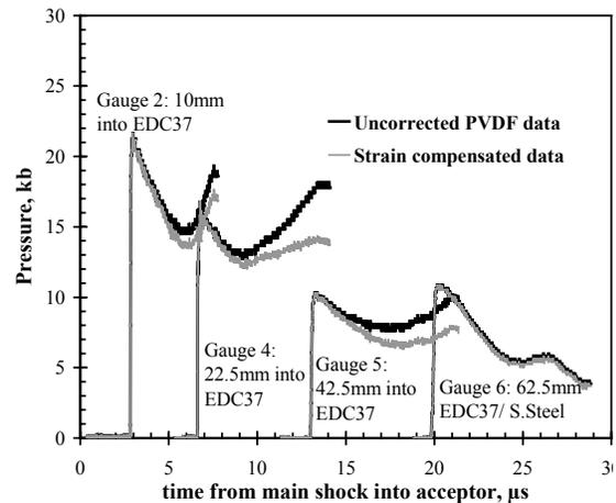
**FIGURE 18. STRAIN COMPENSATION APPLIED TO SI2D/2 RESULTS.**
