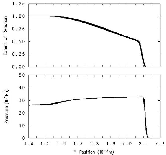
**Figure 3. Pressure and reaction variable profiles every  $0.02 \mu\text{s}$  over the period of  $1.0 \mu\text{s}$  showing steady detonation of an LX-17 charge using Ignition & Growth.**
