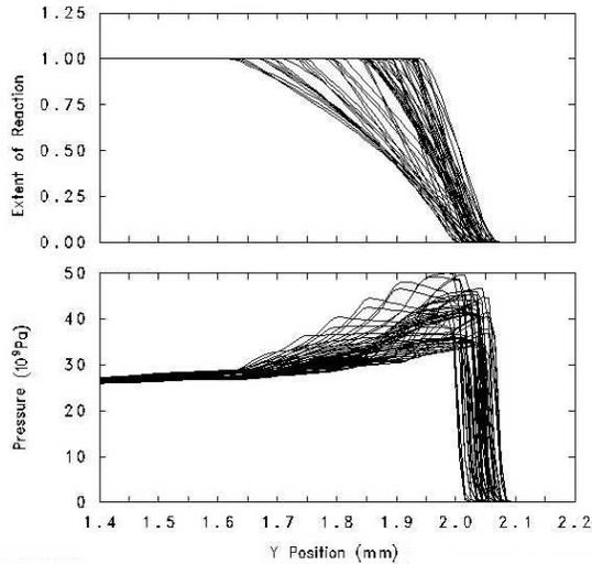
**Figure 2. Pressure and reaction variable profiles every  $0.02 \mu\text{s}$  over the period of  $1.0 \mu\text{s}$  showing periodic unsteadiness in an LX-17 detonation using HVRB.**
