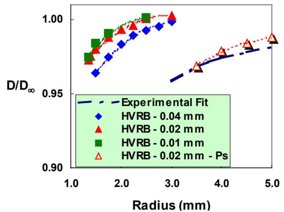
**Figure 5. HVRB predictions of normalized detonation velocity for Octol as a function of charge radius for several computational zone sizes compared with a fit to experimental data.**
