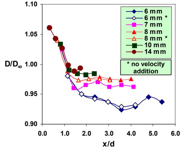
**Figure 4. Normalized detonation velocity as a function of propagation distance in diameters in Composition B3 charges at various diameters.**
