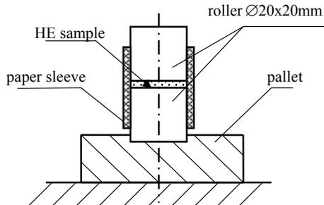
**FIGURE 2. UNIT BM-M FOR HE IMPACT SENSITIVITY TESTS**
