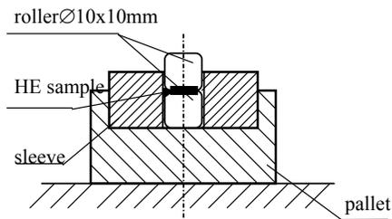
**FIGURE 1. UNIT 1 FOR HE IMPACT SENSITIVITY TESTS**
