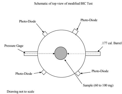
FIGURE 2. TOP VIEW OF BALLISTIC IMPACT EXPERIMENT.
