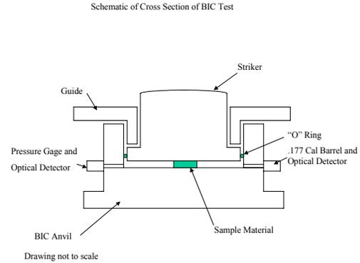
FIGURE 1. SCHEMATIC OF BALLISTIC IMPACT EXPERIMENT.
