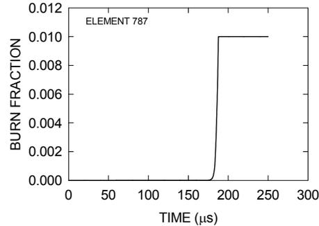
FIGURE 5. BURN FRACTION VS. TIME FOR A CELL NEAR OUTER PERIPHERY OF SAMPLE. APPROXIMATE LOCATION OF CELL IS IN AREA OF LARGEST BURN FRACTION AS SHOWN IN FIG. 4.
