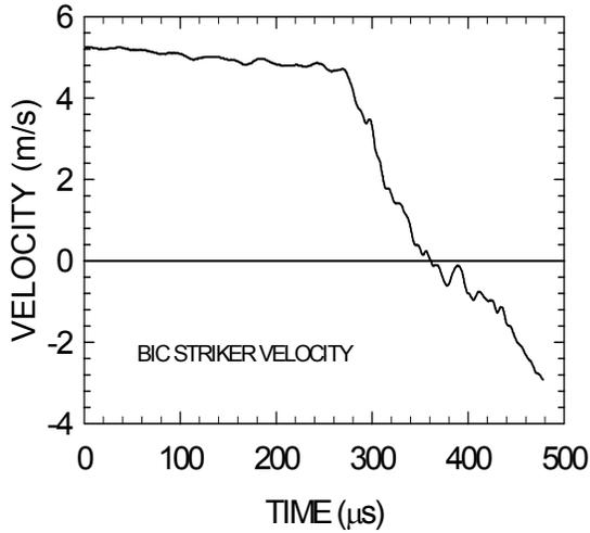
FIGURE 3. STRIKER VELOCITY VS. TIME.
